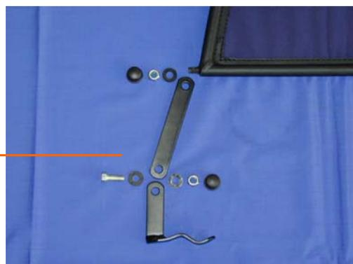
3. Replace the plastic T-bar cover. Now position the wind shield between the two brackets and tighten both ends with nuts provided. Once tighten position into place. Using the black covers, cover the bolts and nuts upon the wind shield brackets.
