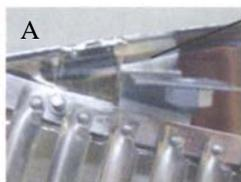
**A.** The original grille shell had a slotted plate brazed in place to attach the upper corners of the grille slat assembly. We have incorporated this design feature into the reproduction.
